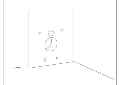
Use the drilling template provided mark and drill holes for the inlet, waste and fixing studding.
